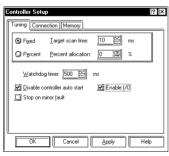
Settings for Using External I/O. In the Pro-Control Editor [Controller] menu, select [Setup] and the [Setup] dialog box will appear.
