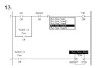
After "Run\_Time\_Timer" is dropped on Rung 2, a pop-up variable window will appear. Double-click on theis window's [Run\_Time\_Timer. Q] variable, which designates the output bit used for "Run\_Time\_Timer."
