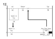
Drag the variable name "Fan" from Rung 2 and drop it onto the Normally-open contact in Rung 3.
